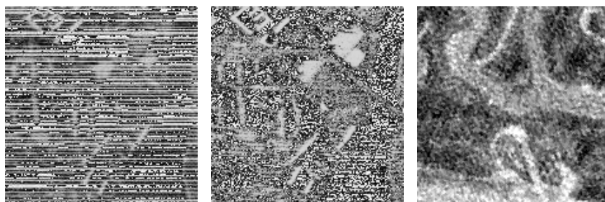
Figure 3.2. Typical noisy channels : respectively Strasbourg (band number 42 and number 59 from DAIS) and Lagoon of Venice (band 45 from DAIS)
