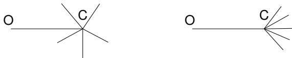
Figure 6. On the left, the normal behaviour in which all the space is used to compute the size of each slice. On the right, a modified behaviour in which a constraint is applied before computing the size of each slice, allowing us to direct the graph in a given way.
